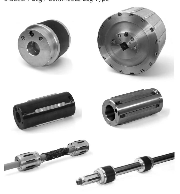
Shaft-mounted expanding chucks expand production abilities in a simple and inexpensive way. They serve as adapters that enable mounting cores with different diameters on a single shaft. They are produced for cores with internal diameter from 70 mm to 350 mm. This is the perfect solution for non-standard diameters.
