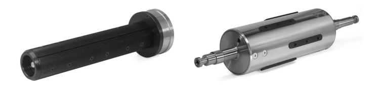
Pneumatic/mechanical shafts combine advantages of mechanical and air operated expanding shafts. Evenly expanding lugs precisely center a roll and an air cylinder ensures stable and firm core clamping. Pumping action is carried out through a valve or rotary union.
