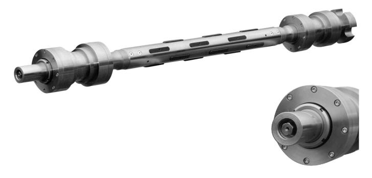
Mechanically expanding shafts ensure perfect centering even very heavy rolls. They are used for rewinding delicate materials or at high speeds of a web. Lugs expand through turning the axially positioned hexagonal head screw. This design makes possible using wrenches of different type, inclusive of air operated ones.
