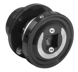
Safety chucks are intended for clamping expanding shafts in a machine. The design ensures safety through automatic closing a chuck at shaft turning. Their main advantage is the possibility of fast refitting a machine.
