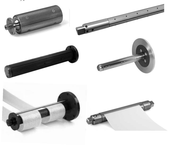
Leaf airshafts combine advantages of lug and continuous lug types. Leaves ensure firm gripping pressure evenly distributed along the entire length and circumference of a core. This is the perfect solution for gripping delicate thin-walled cores. For leaf type airshafts, it is possible to wind a web directly on a shaft without any core.
